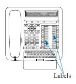
There are two paper labels to enable you to mark the names of correspondents or functions programmed on each group of 10 keys.
